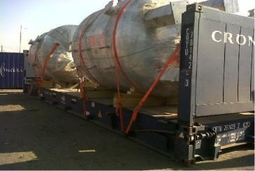
This shipment was loaded with single handling and reduced transit time of 45 days. Combinations of open-top, flat track, 40'ft containers were used to load the shipment.
